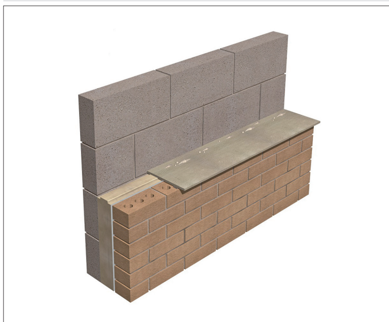
Figure 4 Use of cavity board when cleaning off excess mortar
