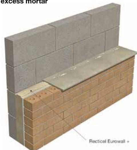
8. To fit around any opening, doors or windows, boards should be cut carefully and accurately to completely fill the spaces for which they are intended, ensuring continuous insulation throughout the wall.
